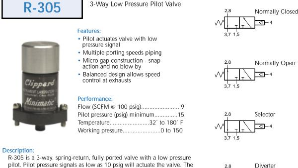
pilot. Pilot pressure signals as low as 10 psig will actuate the valve. The valve can be used normally-OPEN, normally-CLOSED, as a selector or as a diverter. The R-305 may be used in place of an R-301 valve where a lower pilot actuation pressure is desired. It can also be used as a 2-way valve by plugging the exhaust ports.
